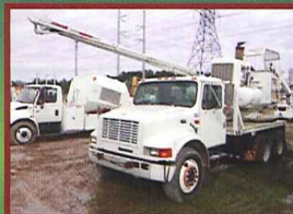
HIGHWAY PRESSURE DIGGER ON 1998 INTERNATIONAL 4900 (JACKSONVILLE, FL)
