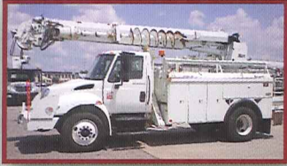
ALTEC DM47-BR DIGGER DERRICK ON 2007 IHC 4300
